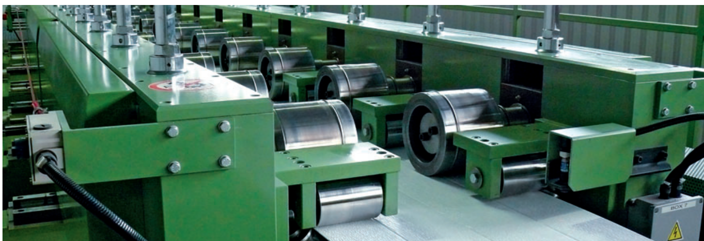
Beginning of panel production – sheet forming
