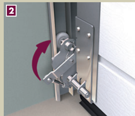
2 Cord break protection protects the door leaf from dropping in the case of carrying ropes being damaged.
